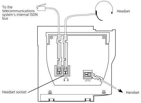
Terminals on the underside of the digital system telephone ST  $\mathbf{25}$
