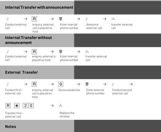
When transferring an external call, you must always seize the outside line by entering "9", even if spontaneous outside line seizure with internal is set on the telephone.
