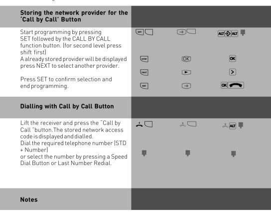
The network access code which has been dialled with the Call By Call button will not be stored in the last number redial.
