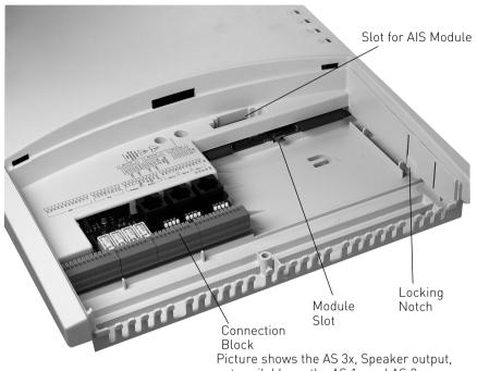
Picture shows the AS 3x, Speaker output, not available on the AS 1x and AS 2x
